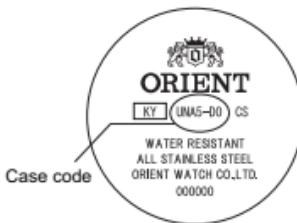
**Example :** When the case code is "UNA5-D0", the caliber number is "UN".
